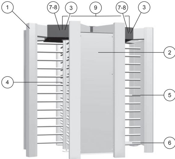
Based on a modular design approach, the 36x full-height turnstile range is available with 3 or 4 arms, manual or motorized, single or double passage versions. The TRS363 manual and TRS368 motorized versions belong to this new generation of full-height turnstiles.
