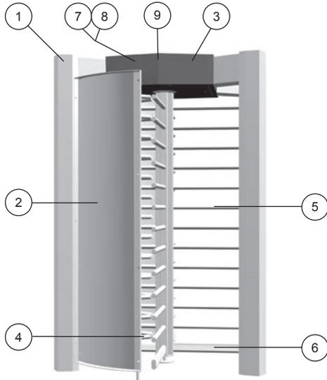
Based on a modular design approach, the 36x full-height turnstile range is available with 3 or 4 arms, manual or motorized, single or double passage versions. The TRS361 manual and TRS366 motorized versions belong to this new generation of full-height turnstiles.
