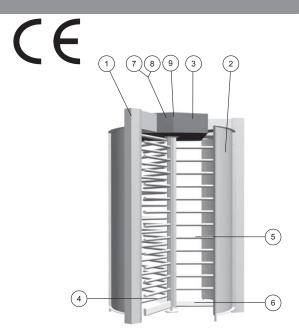
Based on a modular design approach, the 36x full-height turnstile range is available with 3 or 4 arms, manual or motorized, single or double passage versions. The TRS360 manual and TRS365 motorized versions belong to this new generation of full-height turnstiles.
